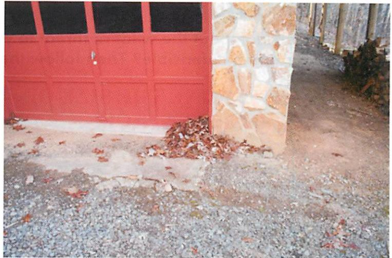
Firebrands and embers will collect in the same places around and on homes and structures during a wildfire, as they do during a windstorm. Looking for these areas and reducing or removing any combustible material from this area will reduce the ignition potential.
